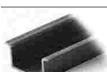
Item no.: 210-114 Steel carrier rail; 35 x 15 mm; 1.5 mm thick; 2 m long; unslotted; similar to EN 60715; silver-colored
