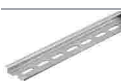
Item no.: 210-115 Steel carrier rail; 35 x 7.5 mm; 1 mm thick; 2 m long; slotted; according to EN 60715; "Hole width 18 mm; silver-colored
