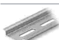
Item no.: 210-112 Steel carrier rail; 35 x 7.5 mm; 1 mm thick; 2 m long; slotted; according to EN 60715; "Hole width 25 mm; silver-colored
