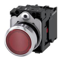
Illuminated pushbutton, 22 mm, round, metal, shiny, red, pushbutton, flat, momentary contact type, with holder, 1NC, LED module with integrated LED 230 V AC, screw terminal, with laser labeling, inscription or symbol Customer-specific selection with SIRIUS ACT configurator (CIN)
