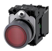
Illuminated pushbutton, 22 mm, round, plastic with metal front ring, red, pushbutton, flat, momentary contact type, with holder, 1NO, LED module with integrated LED 24 V AC/DC, screw terminal, with laser labeling, lower case
