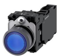
Illuminated pushbutton, 22 mm, round, plastic with metal front ring, blue, pushbutton, flat, momentary contact type, with holder, 1 NO+1 NC, LED module with integrated LED 230 V AC, screw terminal, with laser labeling, upper case and lower case, always upper case at beginning of line
