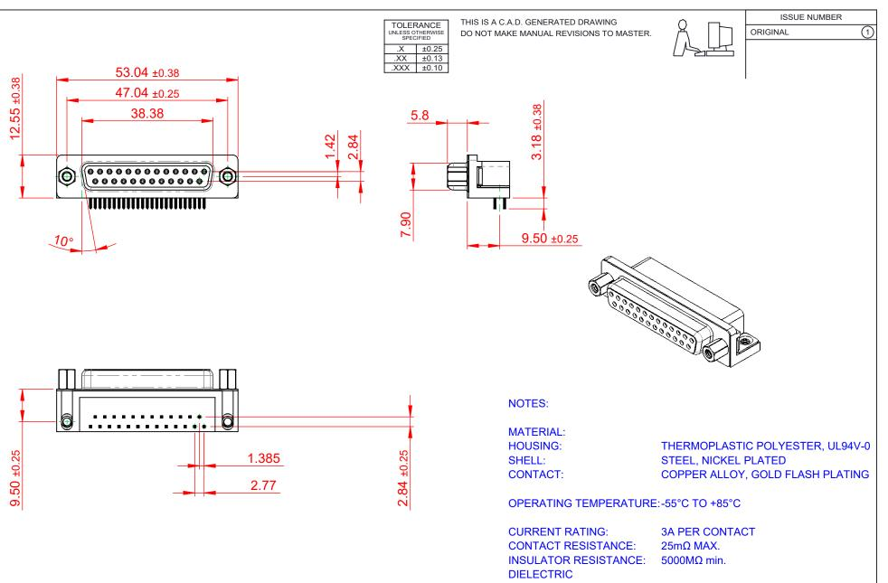
WITHSTANDING VOLTAGE: 1000V AC rms
