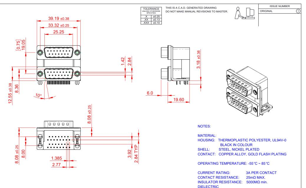
WITHSTANDING VOLTAGE: 1000V AC rms
