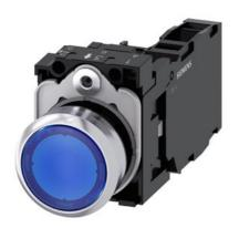
Illuminated pushbutton, 22 mm, round, metal, shiny, blue, pushbutton, flat, momentary contact type, with holder, 1 NO+1 NC, LED module with integrated LED 24 V AC/DC, screw terminal, with laser labeling, symbol number according to, ISO 7000 or IEC 60417
