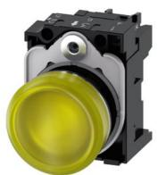
Indicator lights, 22 mm, round, metal, shiny, yellow, lens, smooth, with holder, LED module with integrated LED 110 V AC, screw terminal, with laser labeling, symbol number according to, ISO 7000 or IEC 60417
