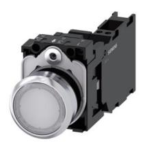
Illuminated pushbutton, 22 mm, round, metal, shiny, white, pushbutton, flat, momentary contact type, with holder, 1 NO+1 NC, LED module with integrated LED 230 V AC, spring-type terminal, Z=20-unit packaging
