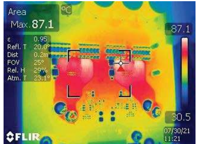
Figure 5. Thermal image showing FET region (back side of the board) temperature at full load with heatsink and 2000 LFM forced air cooling
