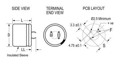
**General Information** Series PEH526 Dielectric Aluminum Electrolytic Description Snap-In, Aluminum Electrolytic RoHS Lead 3 Pin Short Qualifications AEC-Q200 AEC-Q200 Yes Component Weight 24 g Notes Add 0.5mm To D And 1mm To L For Sleeving. 520 Weeks Shelf Life
