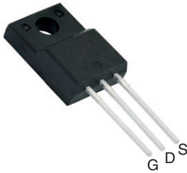
Thin-Lead TO-220 FULLPAK
