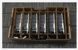
**Step 2:** Two stacks of inner boxes (totaling 12 Modules, all having same voltage bin) are placed inside one outer box:
