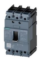
circuit breaker 3VA5 UL frame 125 breaking capacity class S 25kA @ 480 V 3-pole, line protection TM210, FTFM, In=100A overload protection Ir=100A fixed short-circuit protection Ii=10 x In nut keeper kit on both sides
