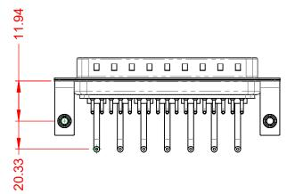
POWER/CO-AX CONTACT RATING: (IF PRESENT) SIGNAL CONTACT CURRENT RATING: 5A PER CONTACT SIGNAL CONTACT RESISTANCE:  $10m\Omega$  MAX.
