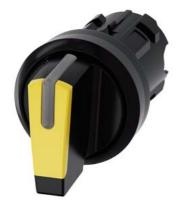
Selector switch, illuminable, 22 mm, round, plastic, yellow, selector switch, short, 3 switch positions I>O<II, momentary contact type, actuating angle 2x45°, 10:30h/12h/13:30h, with laser labeling, inscription or symbol Customer-specific selection with SIRIUS ACT configurator (CIN)
