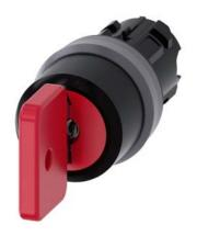
Key-operated switch O.M.R, 22 mm, round, plastic with metal front ring, lock number 73037, red, with 2 keys, 3 switch positions I>O<II, momentary contact type, actuating angle 2x45°, 10:30h/12h/13:30h, key removal O, Z=50-unit packaging
