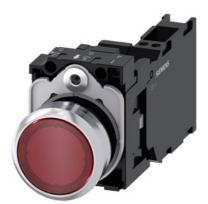
Illuminated pushbutton, 22 mm, round, metal, shiny, red, pushbutton, flat, momentary contact type, with holder, 1 NO+1 NC, LED module with integrated LED 24 V AC/DC, spring-type terminal, with laser labeling, upper case and lower case, Always upper case at the beginning of the word
