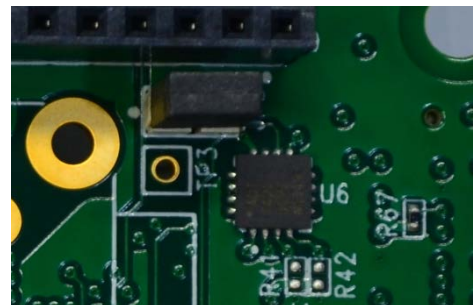
Figure 7. I 2 C Temperature Circuit
