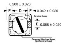
**HRSPD74** Height Dimension 'C' 0.198 Inches Max (5.03 mm Max) **HRSPD74** Terminal Dimensions  $0.190 \pm 0.005$  'D' (in) by  $0.100 \pm 0.010$  'F' (in)
