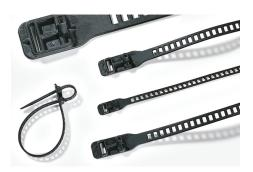
Manufactured from a soft, tear-resistant thermoplastic polyurethane these ties have several unique features: strong, yet elastic, and suitable for temperatures as low as -20 degrees C. The SOFTFIX ties are releasable and reusable which is ideal for bundling cables in temporary applications such as musical events, theatres etc.
