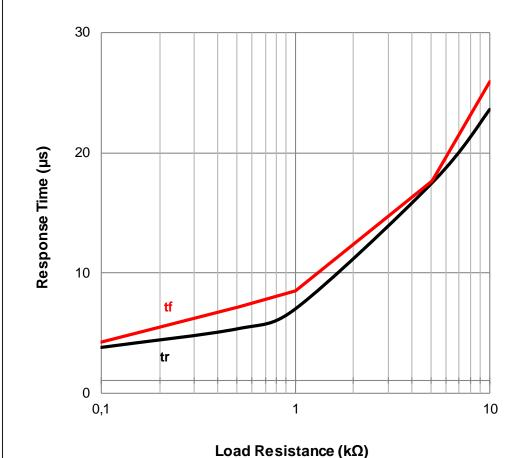
Relative to  $I_c = 1 \text{mA}$ ;  $TA = 25^{\circ}\text{C}$ Testcondition:  $I_c = 2 \text{mA}$ ;  $V_{cF} = 2 \text{V}$ ;  $TA = 25^{\circ}\text{C}$
