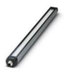
LED machine light, 24 V DC, emission angle 85 °/95 °, color temperature 5000 K, length 540 mm, diameter 40 mm, M12 connector, Light housing: Anodized aluminum, Pane: Single-pane safety glass (ESG, thermally toughened float glass), pivoting, resistant to coolants and lubricants, can be switched in series
