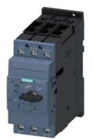
Circuit breaker size S2 for motor protection, Class 20 A-release 12...17 A N-release 260 A screw terminal Standard switching capacity
