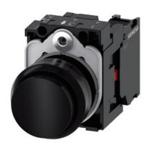
Pushbutton, 22 mm, round, plastic, black, pushbutton, raised, momentary contact type, with holder 1 NC, screw terminal, with laser labeling, upper case and lower case, always upper case at the beginning of the word
