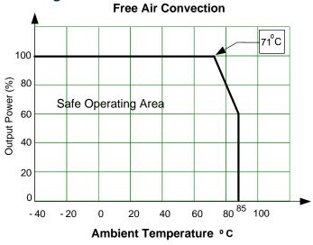
NOTE: With air convection speed of 0.8m/sec
