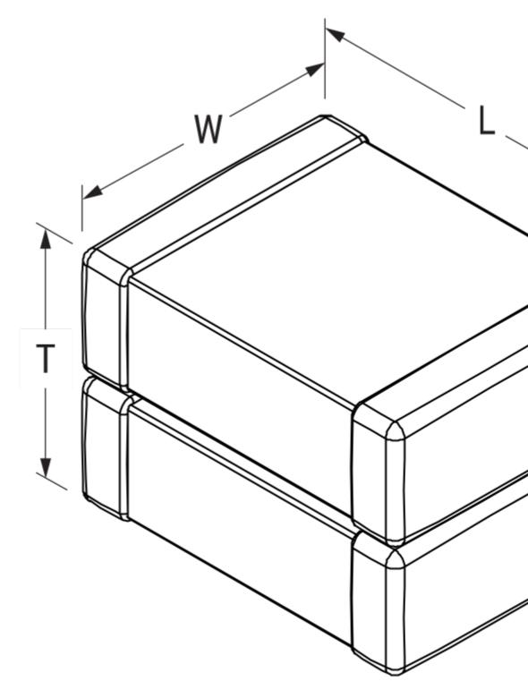
Click here for the 3D model. **Dimensions** L 5.9mm +/-0.75mm W 5mm +/-0.4mm T 3.1mm +/-0.3mm
