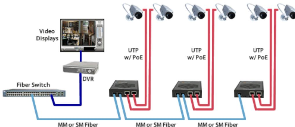
A second option is to have redundant fiber links for installations requiring fiber facility protection. There is an active fiber port and a protection fiber port that can support a fiber failure switchover of less than 50 milliseconds. The PoE+ media converter supplies power
