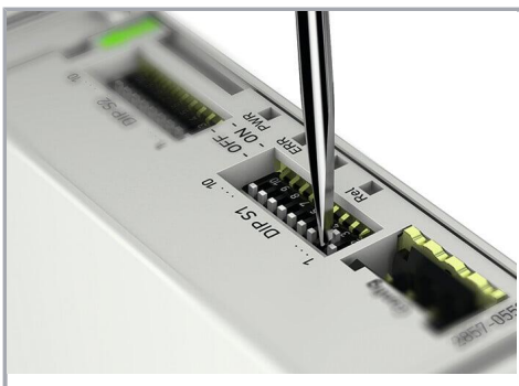
Configuration via DIP switch
