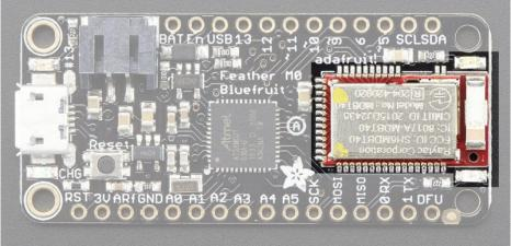
Since not all pins can be brought out to breakouts, due to the small size of the Feather, we use these to control the BLE module
