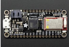
Bluefruit Micro or Feather 32u4 Bluefruit If you have a Bluefruit Micro or Feather 32u4 Bluefruit LE then you have an ATmega32u4 chip with Hardware SPI, CS = 8, IRQ = 7, RST = 4
