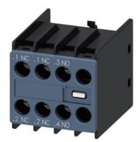
Auxiliary switch on the front, 1 NO + 2 NC Current path 1 NC, 1 NC, 1 NO for 3RH and 3RT screw terminal .1/.2, .1/.2, .3/.4
