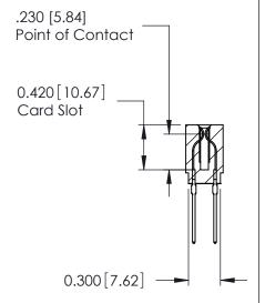
ACAD REFERENCE NO. 725-ENG MASTER 725 Series Ultra-Mate Card Edge Connector - Press Fit SEGAHOM:3A:9A DRAWN: J.LEE Part Number: 725-048-545-201 CHECKED: DATE: SCALE: **EDAC INC** SHEET 1 OF 1 THESE DRAWINGS AND SPECIFICATIONS ARE THE PROPERTY OF EDAC INC., AND TORONTO, ONTARIO SHALL NOT BE REPRODUCED, OR COPIED DRAWING NUMBER **ISSUE** CANADA OR USED AS THE BASIS FOR THE 725-ENG MASTER MANUFACTURE OR SALE OF APPARATUS YOUR CONNECTION TO QUALITY & SERVICE WITHOUT WRITTEN PERMISSION.
