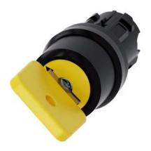
Key-operated switch O.M.R, 22 mm, round, plastic, lock number 73033, yellow, with 2 keys, 2 switch positions O-I, latching, actuating angle 90°, 10:30h/13:30h, key removal O+I, with laser labeling, lower case
