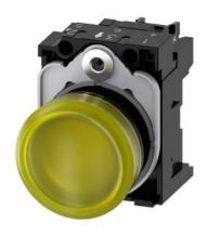
Indicator lights, 22 mm, round, plastic, yellow, lens, smooth, with holder, LED module, with integrated LED 24 V AC/DC, screw terminal, with laser labeling, inscription or symbol Customer-specific selection with SIRIUS ACT configurator (CIN)
