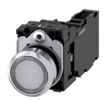
Illuminated pushbutton, 22 mm, round, metal, shiny, clear, pushbutton, flat, momentary contact type, with holder, 1 NO+1 NC, LED module with integrated LED 110 V AC, screw terminal, with laser labeling, symbol number according to, ISO 7000 or IEC 60417
