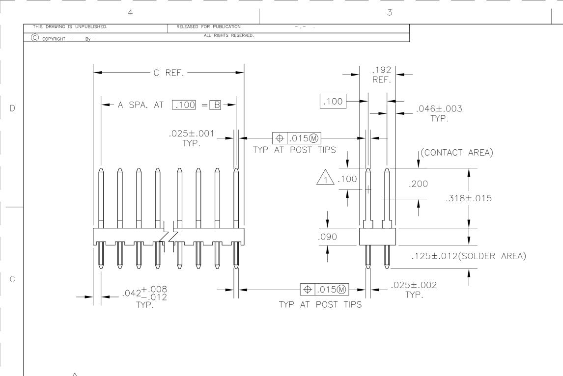
1 POINT OF MEASUREMENT FOR PLATING THICKNESS
