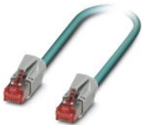
Assembled Ethernet cable, CAT5e, shielded, 2-pair, AWG 26 stranded (7-wire), RAL 5021 (water blue), RJ45 connector/IP20 on RJ45 connector/IP20, line, length 0.3 m
