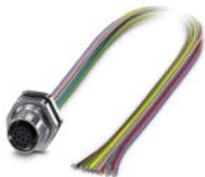
Flush-type connector, Universal, 17-position, Socket, M12, A-coded, Rear mounting, M16 x 1.5, Individual wires, cable length: 0.5 m
