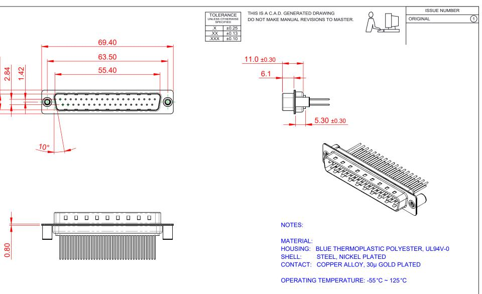
**CURRENT RATING: 5A PER CONTACT** CONTACT RESISTANCE:  $25m\Omega$  MAX. INSULATOR RESISTANCE: 5000MΩ min. DIELECTRIC WITHSTANDING VOLTAGE: 1000V AC rms
