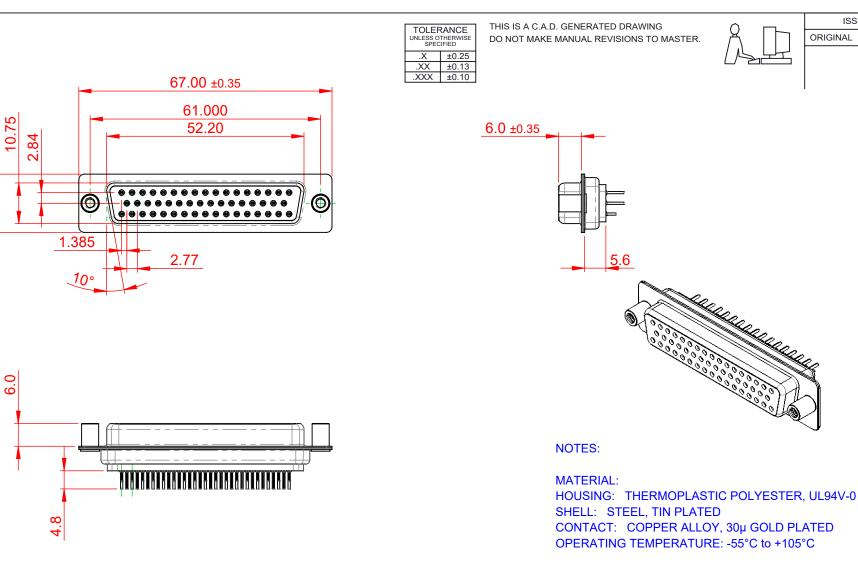
CURRENT RATING: 3A PER CONTACT CONTACT RESISTANCE: 25mQ MAX. INSULATOR RESISTANCE: 5000MΩ min. DIELECTRIC WITHSTANDING VOLTAGE: 1000V AC rms
