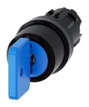
Key-operated switch O.M.R, 22 mm, round, plastic, lock number 73038, blue, with 2 keys, 3 switch positions I-O-II, latching, actuating angle 2x45°, 10:30h/12h/13:30h, key removal O, with laser labeling, upper case and lower case, always upper case at the beginning of the word
