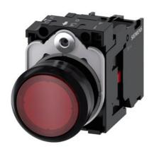
Illuminated pushbutton, 22 mm, round, plastic, red, pushbutton, flat, momentary contact type, with holder, 1NC, LED module with integrated LED 230 V AC, screw terminal, with laser labeling, inscription or symbol Customer-specific selection with SIRIUS ACT configurator (CIN)
