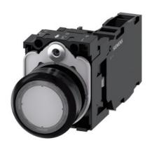
Illuminated pushbutton, 22 mm, round, plastic, clear, pushbutton, flat, momentary contact type, with holder, 1 NO+1 NC, LED module with integrated LED 24 V AC/DC, screw terminal, Z=20-unit packaging
