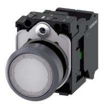
Illuminated pushbutton, 22 mm, round, plastic with metal front ring, white, pushbutton, flat, momentary contact type, with holder, 1NO, LED module with integrated LED 24 V AC/DC, spring-type terminal, with laser labeling, lower case
