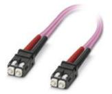
Assembled FO cable, zip cord cable, multi-mode fiberglass 50/125  $\mu$ m, OM4, plug: SC-RJ/SC-RJ, degree of protection: IP20, for installation in cable ducts or control cabinets, length: 1 m
