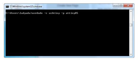
Now plug in the Trinket into the computer's USB port and/or press the reset button to enter the bootloader. You should see the red LED pulsing. Now press return, you should get the same response as shown here:
