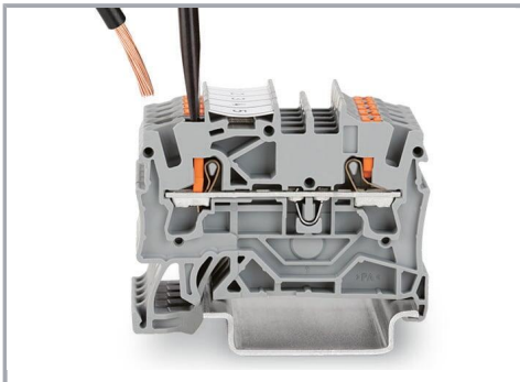
Insert fine-stranded conductors via operating tool.
