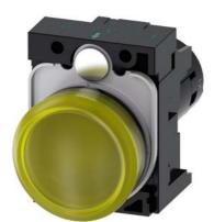
Indicator lights, compact, 22 mm, round, plastic, yellow, lens, smooth, with holder, Operating voltage 24 V AC/DC, screw terminal
