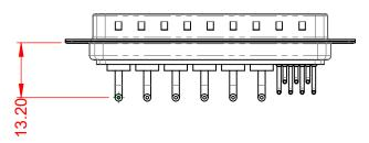
POWER/CO-AX CONTACT RATING: (IF PRESENT) SIGNAL CONTACT CURRENT RATING: 5A PER CONTACT SIGNAL CONTACT RESISTANCE:  $10m\Omega$  MAX. **INSULATOR RESISTANCE:** 5000MΩ min. DIELECTRIC
