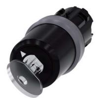
key-operated switch Siemens, 22 mm, round, plastic with metal front ring, lock no. LSG1, with 2 keys, 2 switch positions O<I, momentary contact type, actuating angle 45°, 10:30h/12h, key removal O, Z=50-unit packaging
